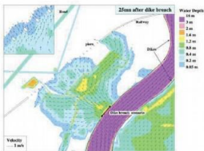
Overflow subsequent to an embankment failure
